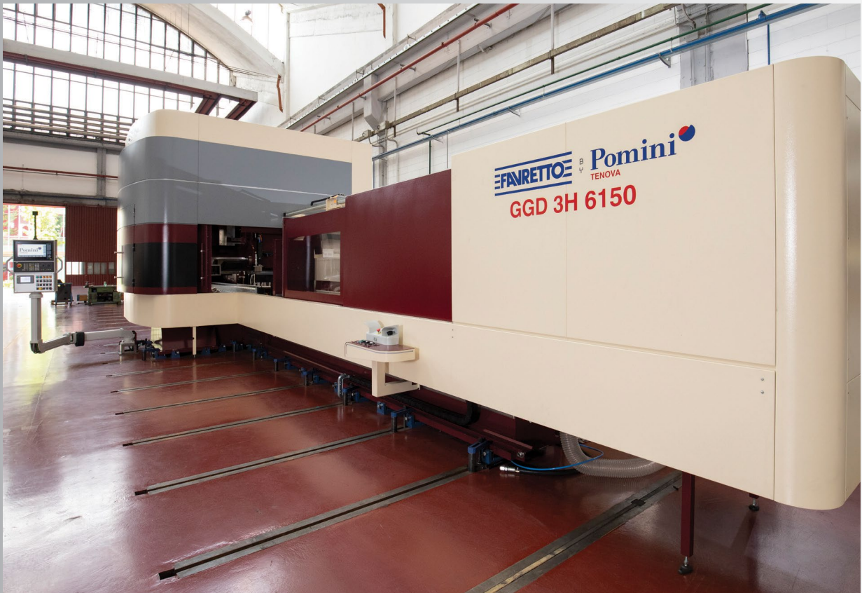
Large portal machines with fixed crossrail for grinding Linear Roller and Linear Ball Guideways.
